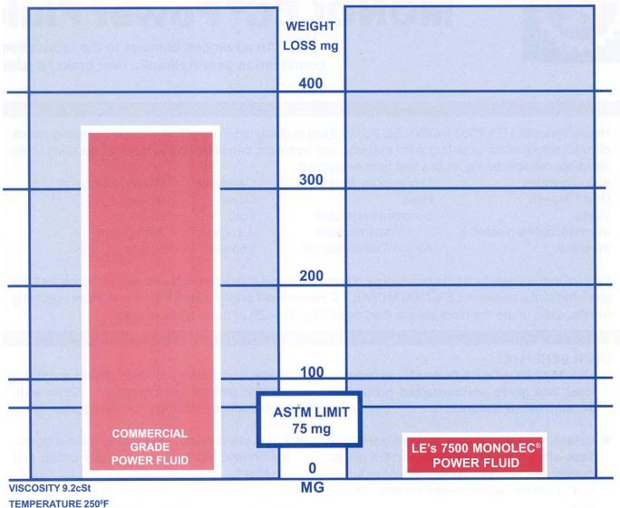
The graph above shows the results of the ASTM D-4998 Gear Wear Test which utilizes a modified FZG apparatus that operates at gear loadings of 284,000 psi (10<sup>th</sup> load stage), speeds of 100 rpm, and a temperature of 121°C (250°F) for a duration of 10 hours. At the end of the test, the gears are removed, weighed and visually inspected.
